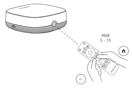
Turn on the TV and the streaming box and follow the instructions on the screen to pair the remote control.
